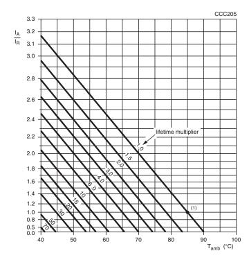
$I_A$  = actual ripple current at 120Hz  $I_R$  = rated ripple current at 120 Hz, 85 °C  $^{(1)}$  useful life at 85 °C and  $I_R$  applied: 1500 h
