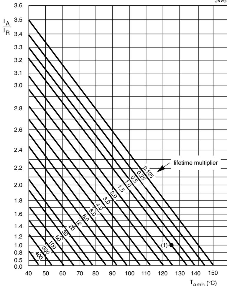
$I_A$  = actual ripple current at 10 kHz
