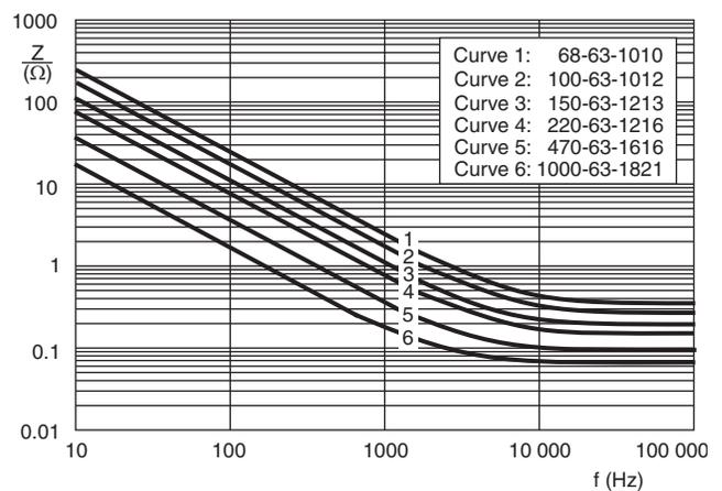
Fig. 9 - Typical impedance as a function of frequency
