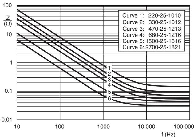
Fig. 8 - Typical impedance as a function of frequency
