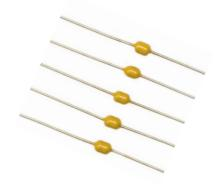
NOVACAP Axial Leaded Capacitors are available in COG, X7R and X8R characteristics. Conformal coating and lead mounting provide a rugged configuration for optimum performance, with high capacitance efficiency per KV rating. Units are designed for commercial/industrial use to 2 KV, with application in power supply and voltage multiplier circuits. High reliability versions with restricted capacitance ranges are also available. Please refer to other NOVACAP literature, or consult the factory.
