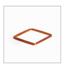
A special version of enamelled wire is self-bond enamelled wire. Its adhesive properties are activated thermally or by a solvent. After activation, the individual windings bond into a self-sustaining coil. The use of self-bond enamelled wire gives a range of cost and manufacturing benefits due to the savings made on coil forms, adhesive tape, casting compounds and impregnation. We are able to manufacture these coils in a range of different sizes and shapes.
