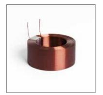
Air-core coils are inductive components without a ferromagnetic core and therefore have relatively low inductance. The magnetisation curve is linear. Air-core coils feature no magnetic saturation compared to coils with magnetic cores. Without a core, magnetic paths cannot be guided resulting in a high level of magnetic flux leakage.
