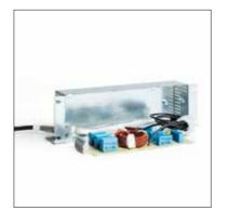
Line filters are effective in limiting electromagnetic interference produced, for example, by inverter drives. They are located in the electrical supply and therefore minimise low-frequency interference while smoothing out current flows. Special components then filter out high-frequency components.
