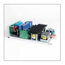
Power supplies with regulating capabilities are known as switch mode power supply units. These convert direct (including non-regulated) voltage into regulated direct voltage with electronic circuits switching between input voltages and electrical earths at high frequencies (e.g. 50 kHz). A connected inductor and capacitor filter the rectangular wave voltage and direct voltage emerges at the output. A control circuit ensures that the duty cycle is set to produce the required output voltage.
