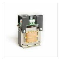
Mains transformers have the task of transforming input voltages to the required output voltages. A mains transformer has two separate coils. Version sizes range from single-phase to 1 kVA and multi-phase up to 5 kVA. Coil types are available in solder plug, clamp and bracket versions.
