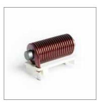
Output chokes are connected in front of inverters to minimise their negative effects. Voltage spikes from in-line motors are reduced to increase motor service life by diminishing insulation loads.
