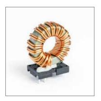
PFC (power factor correction) chokes are used to significantly reduce mains harmonic distortions – generally in line with the mains supply in SMPS components. They function either passively for mains frequency on a laminated transformer core or as a storage choke with a powder core in an active PFC switch mode of 10 to 100 kHz.
