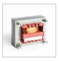
Safety transformers output secondary low voltages for SEL and PELV circuits. A safety transformer has 2 separate coils which may not hold in excess of 50 VAC and 120 VDC when idling. Version sizes range from single-phase to 10 kVA and multi-phase up to 16 kVA. Coil types are available in solder plug, clamp and bracket versions.
