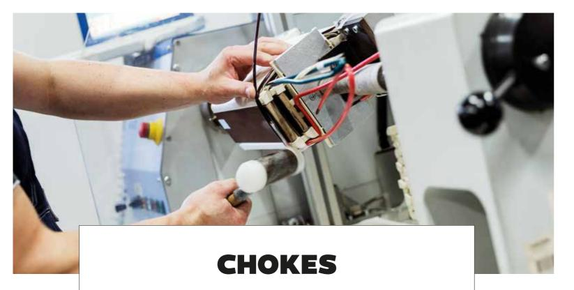
Choke inductors are coils for blocking electrical currents. They can buffer energy, modify impedance and filter.
