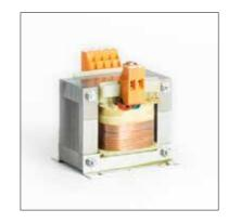
Through their additional ±5 % tappings, control transformers equalise mains undervoltages and overvoltages and are able to suppress short circuit in case of malfunction to permit auxiliary circuits to function unearthed. A control transformer has two separate coils. Version sizes range from single-phased up to 25 kVA and multi-phased up to 40 kVA. Coil types are available in solder plug, clamp and bracket versions.
