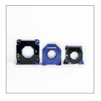
We use our know-how to produce current sensors with the Hall effect at different sizes and with different powers. Current sensors equipped with the Hall effect are generally sensitive to temperatures making temperature compensation necessary. Very high currents – including short-term high input surge currents – can lead to the core material becoming magnetised. Measurement errors and/or zero offsets then result due to remanence.
