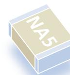
Two position alpha numeric marking is available on chip sizes 0805 through 3333. The marking denotes retma value and significant figures of capacitance (see table) eg: A5 = 100,000pF.
